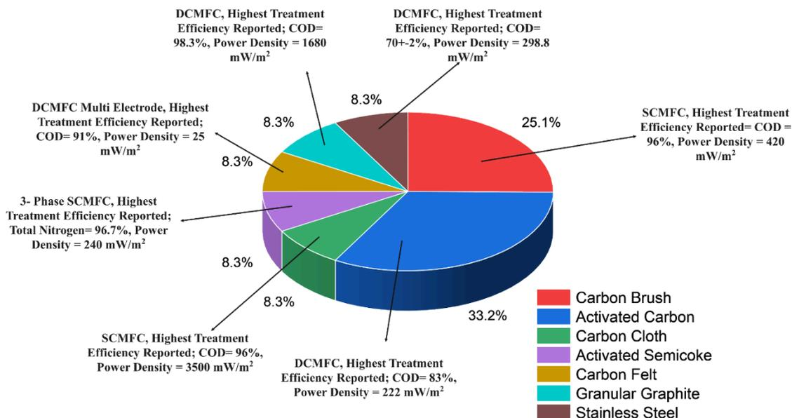
Figure 8. Material Analysis of Industrial MFCs<sup>[42][24][10][11][27][60][8][44]</sup>.
