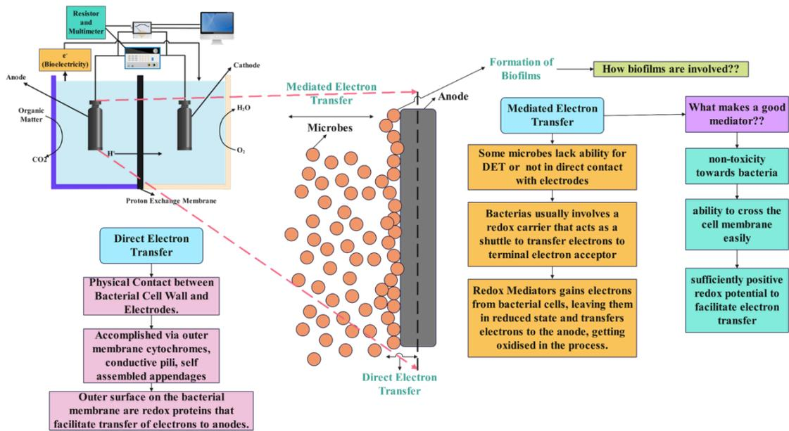
Figure 9. Biofilm mechanism for electron transfer in Microbial Fuel Cell<sup>[75][76][77]</sup>.
