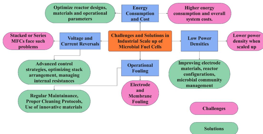
Figure 7. Challenges and Solutions in Industrial Scale-Up of Microbial Fuel Cells<sup>[66][67][68]</sup>.
