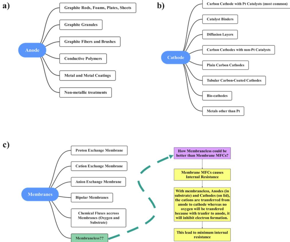
Figure 3. Primary Composition of Materials in Microbial Fuel Cells<sup>[24][25][26][27][28][29]</sup>.
