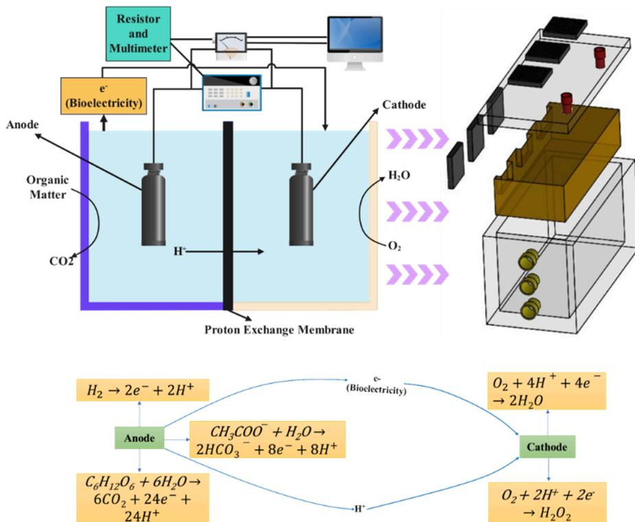
Figure 1. Principal Framework of Microbial Fuel Cells<sup>[5][4]</sup>.
