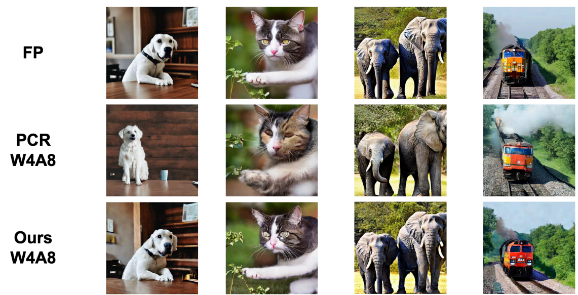
Figure 11. Comparison between the floating-point model and quantized models, using PNDM scheduler, 25 steps.
