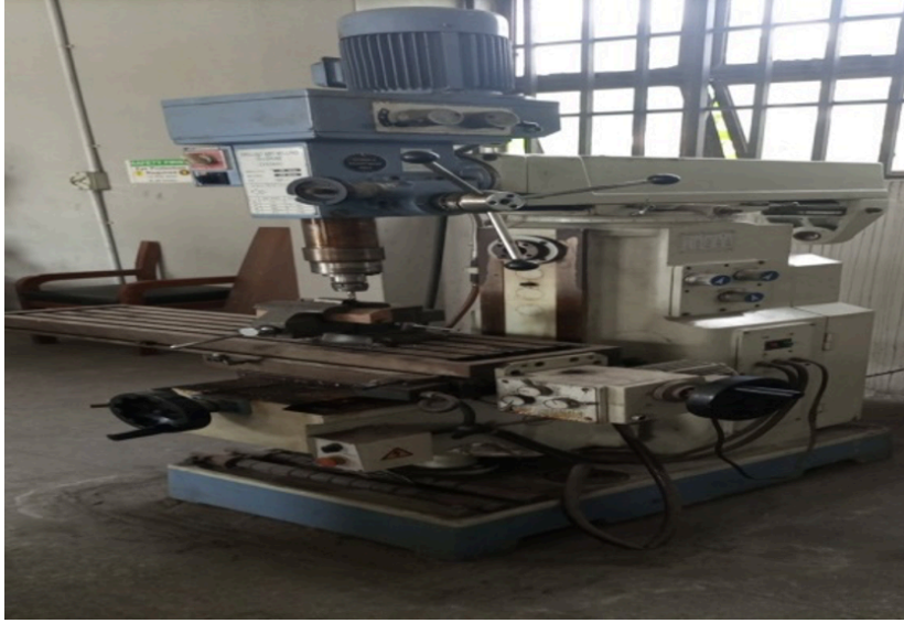
Figure 1. ZX6350C milling machine and workpiece.
