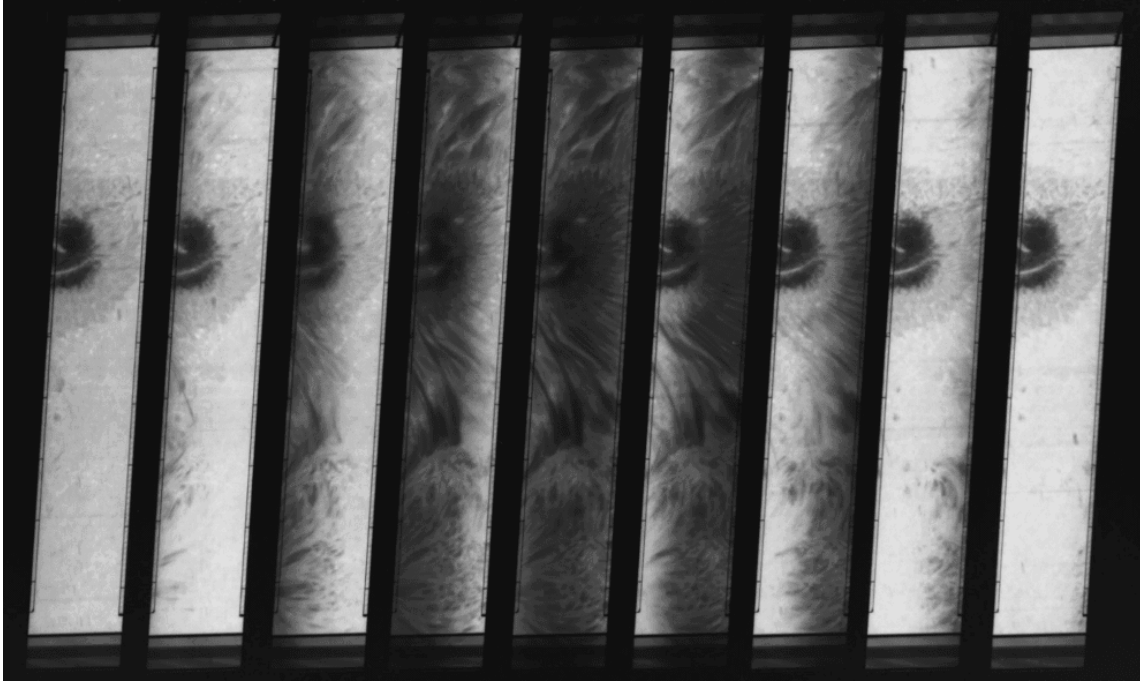
Figure 35. The MSDP of the VTT at Tenerife in H\alpha . The wavelength shift between two consecutive channels is \Delta\lambda = 0.3 \text{ \AA} ; it is governed by the step s (in mm) of the multi-slit of the slicer. At abscissa x inside channel number n , the wavelength is \lambda(x) = \lambda_0 + x/d + n \Delta\lambda , where d is the dispersion of the spectrograph (mm/ \text{\AA} ) and \Delta\lambda = s/d . If w is the width of the rectangular entrance window (in mm), the wavelength variation inside each channel is w/d . Hence, channels are not monochromatic. Courtesy OP.
