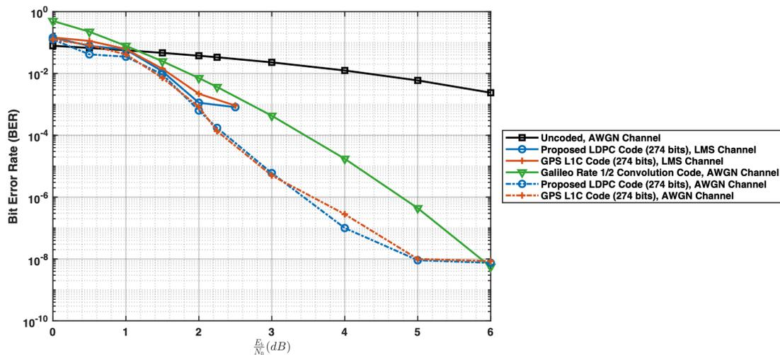
Figure 5. BER performance comparison of proposed QC-LDPC codes ( $m = 274$ ), GPS L1C LDPC codes ( $m = 274$ ), and Galileo 1/2 convolutional codes for AWGN and LMS channels.
