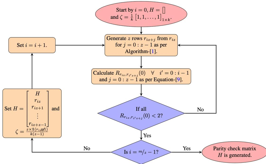
**Figure 2.** Algorithm for Parity Check Matrix generation. Here the function  $\mathbb{1}$  is a standard indicator function which is 1 when the argument is True, else 0.
