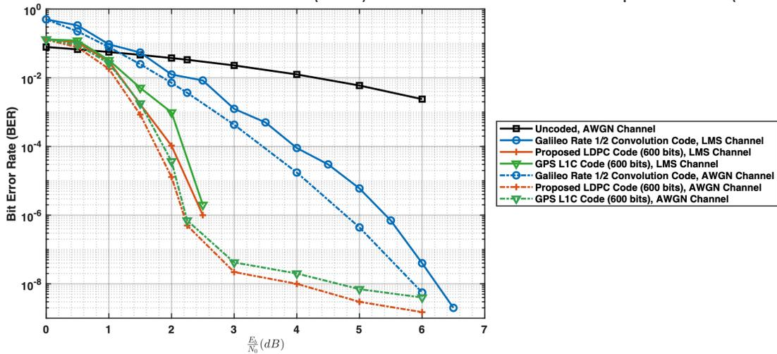
Figure 4. BER performance comparison of proposed QC-LDPC codes ( $m = 600$ ), GPS L1C LDPC codes ( $m = 600$ ), and Galileo 1/2 convolutional codes for AWGN and LMS channels.
