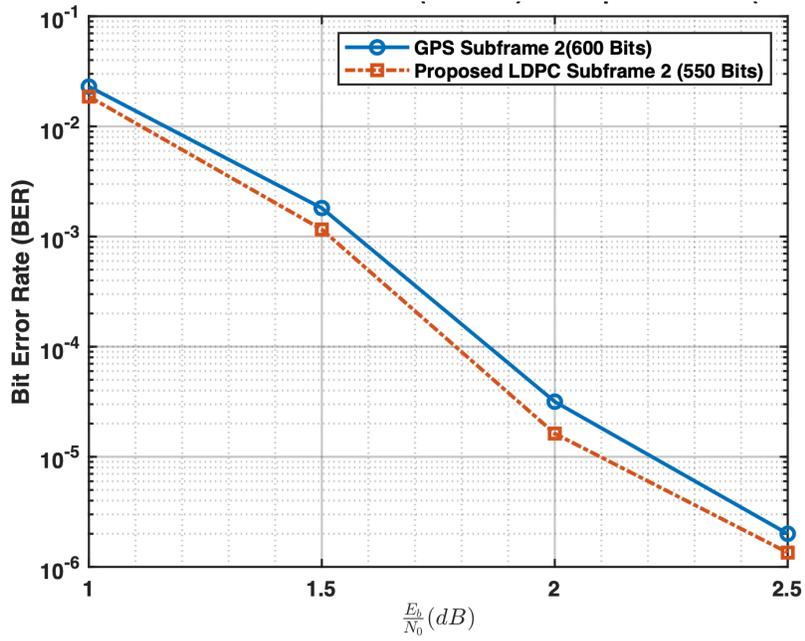
Figure 6. BER performance comparison of proposed QC-LDPC codes ( $m = 550$ ) and GPS LIC LDPC codes ( $m = 600$ ).
