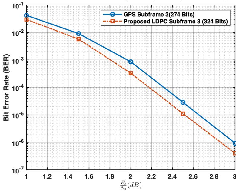
Figure 7. BER performance comparison of proposed QC-LDPC codes ( $m = 324$ ), and GPS LIC LDPC codes ( $m = 274$ ).
