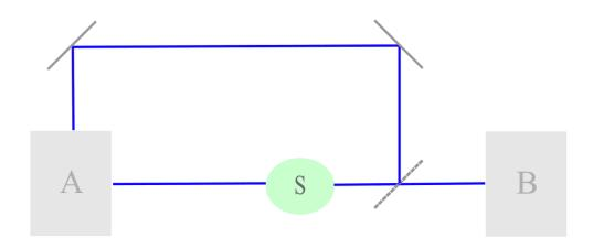
The above diagram illustrates this configuration (where S represents the source, A and B the stations of  $O_1$  and  $O_2$ , and the dashed and solid lines the half and fully silvered mirrors respectively). The evolution of the spin- $\frac{1}{2}$  particle of  $S_2$  is given by the following:
