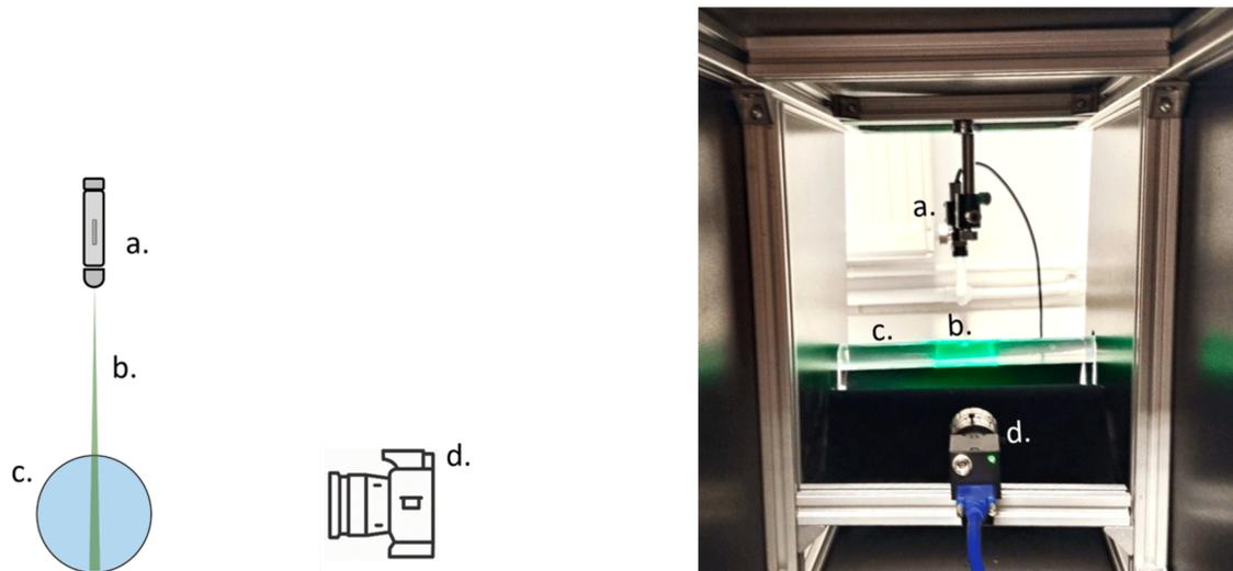
**Figure 2.** 2-D diagram of the lateral view of streak visualization setup (left) and picture of the actual streak visualization system (right) for streak-angle velocimetry. (a) laser, (b) laser sheet, (c) glass pipe, and (d) camera and lens.
