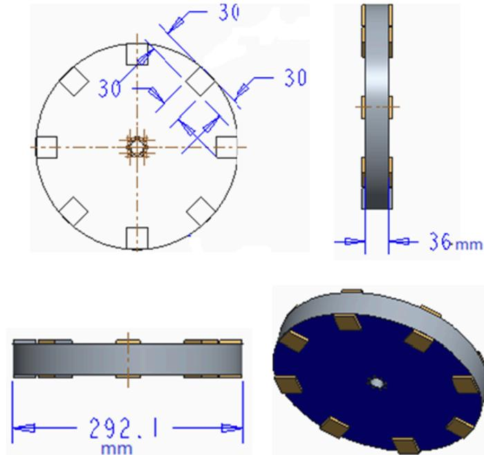
Figure 3. Rotor design
