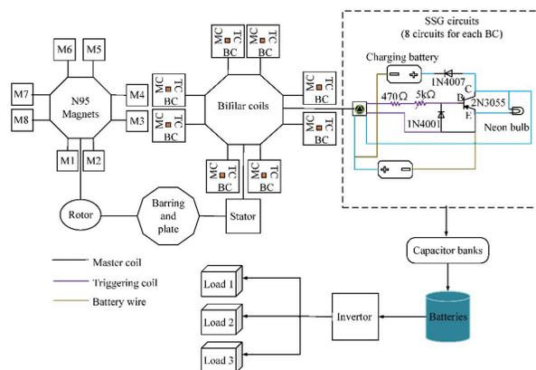
Figure 8. Proposed MFEg's schematic
