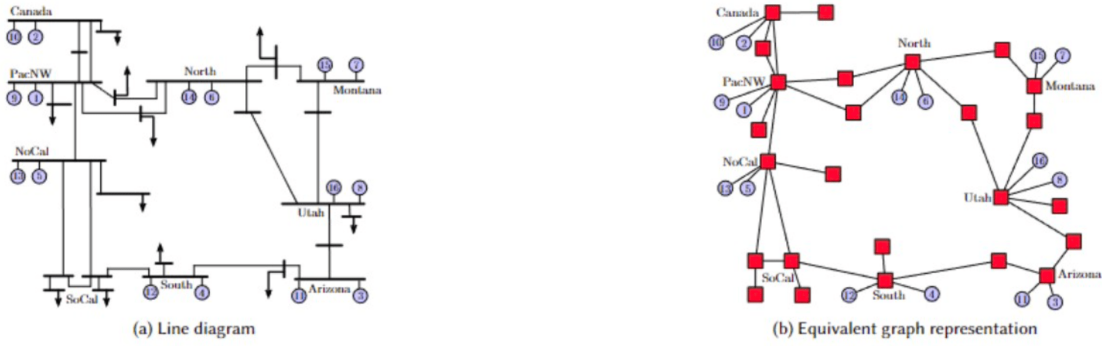
Figure 2. The power network
