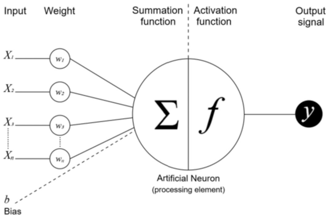
**Figure 2.** A schematic representation of an artificial neuron, illustrating how weighted inputs are summed and passed through an activation function to produce an output signal, forming the basis of neural network computations.
