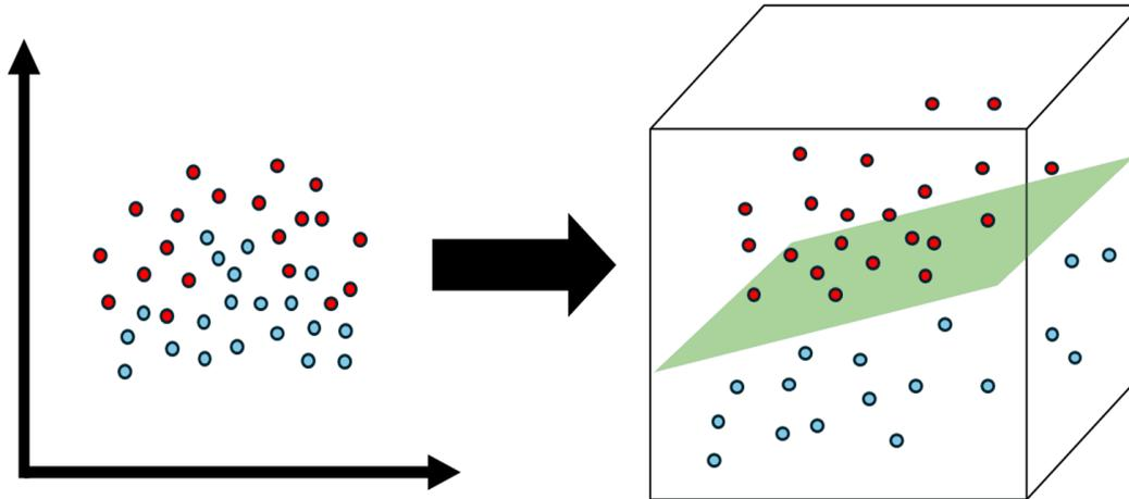
**Figure 4.** A conceptual illustration of Support Vector Machine (SVM) modeling, showing how data is transformed into a higher-dimensional space for optimal separation. The left side depicts data points in two dimensions, while the right side illustrates the resulting hyperplane (green) that separates the classes in a multi-dimensional space, demonstrating SVM's classification mechanism.
