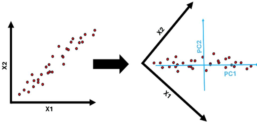
**Figure 5.** A representation of Principal Component Analysis for a two-dimensional system, illustrating how data points are transformed from the original coordinate space ( $X_1, X_2$ ) into a new axis system defined by principal components ( $PC_1, PC_2$ ). The transformation maximizes variance along  $PC_1$ , enabling dimensionality reduction while preserving key data patterns.
