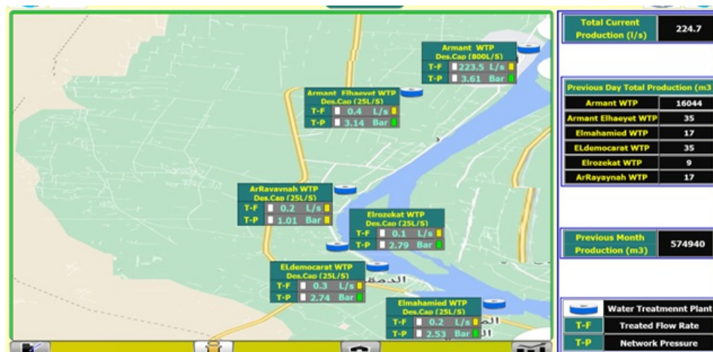
Fig. 1. SCADA Application to monitor water flow and pressure.
