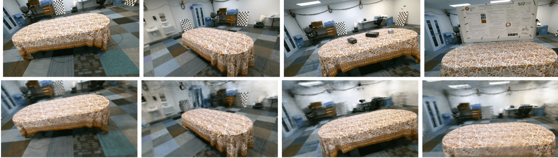
Figure 6. Comparison of NeRF-rendered images to ground truth under normal / minor-change / large-change environments. The top row displays captured images from the closest camera frame, while the second row showcases rendered images at the same positions and orientations. Columns correspond to Table 3-6, progressing from left to right.
