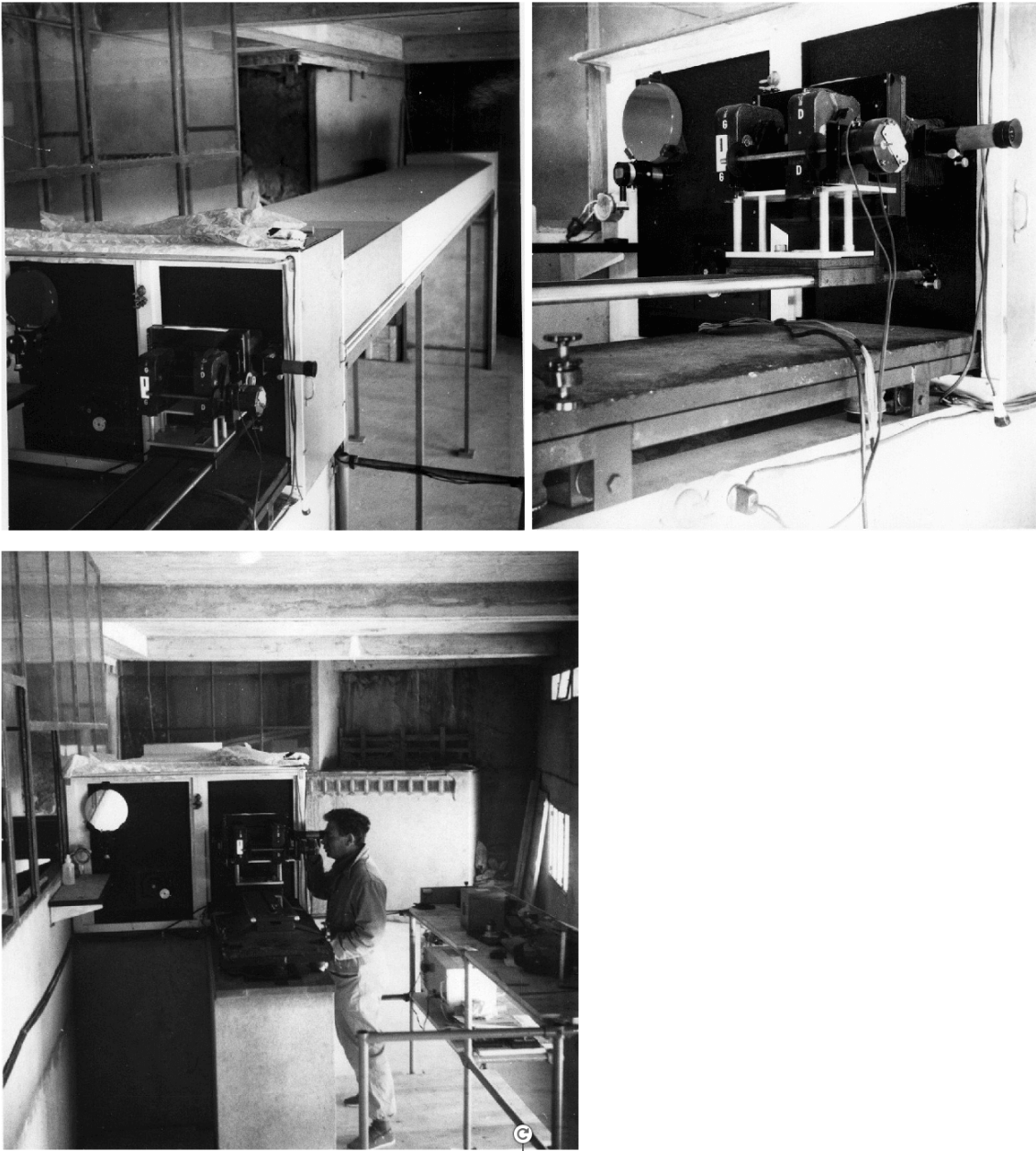
Figure 17. Top: the spectrograph exit with two motorized 35 mm cameras in the spectrum and the eye piece for adjustments. The M3 2X magnifier mirror is visible. The slit is just below the M3. Courtesy OP. Bottom: Roger Servajean at the eye piece in the spectrum. Courtesy OP.
